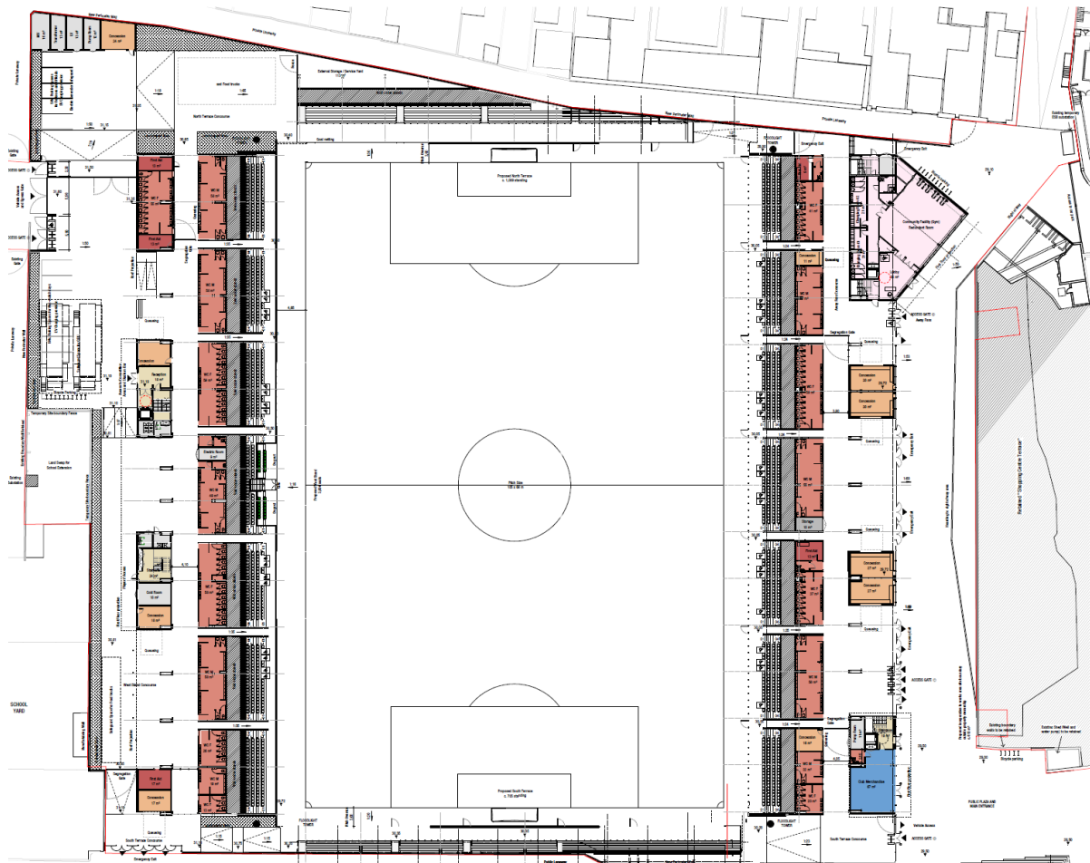
General Ground floor plan, showing concourses, and spectator facilities under stands, Community centre building located in top right corner.
